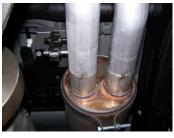
**4.** Slide muffler #B onto head pipe #A 1½"-2" with the louvers facing towards the converter. Use a jack stand to support the muffler. Use clamp #I to secure the muffler to the head pipe. Do not tighten. Outlets will be on the bottom. Install band clamp #J onto muffler. Insert hanger on band clamp into rubber grommets. Use bolt kit provided. Do not tighten.
