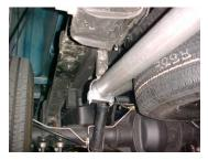
7. Install tail pipe hangers #H onto end of tail pipes using clamp #G. There will be about a 2" hole above the end of both tail pipes on the frame to bolt the hangers. Do not tighten.
