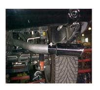
INSTALL YOUR STAINLESS STEEL TIPS. TO CLEAN TIPS USE ANY STAINLESS OR ALUMINUM CLEANER. NOW GO BACK AND TIGHTEN ALL NUTS, BOLTS AND CLAMPS STARTING FROM THE FRONT AND WORKING BACK.
