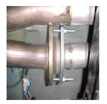
BOLT PASSENGER SIDE HEADPIPE # A USING HARDWARE KIT # L. DO NOT TIGHTEN. INSERT HANGER INTO RUBBER GROMMET, NEXT SLIP DRIVER SIDE HEADPIPE # B ONTO FACTORY PIPE USE CLAMP # G TO SECURE. DO NOT TIGHTEN.
