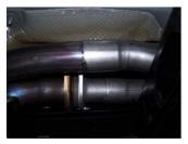
2. Install passenger head pipe #A onto stock Y-pipe with bolt kit #M. Use a jack stand to support the headpipe. DO NOT TIGHTEN. Insert welded hanger into rubber grommet. Next install driver headpipe #B onto the factory pipe, secure with clamp #H. DO NOT TIGHTEN.
