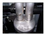
6. Install passenger tailpipe #E onto muffler 1½"-2" secure using clamp #H. DO NOT TIGHTEN. Insert welded hanger into rubber grommet.
