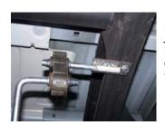
3. Attach rear hanger #H to frame just in front of crossmember. DO NOT TIGHTEN. Attach a rubber grommet off the stock hanger from the rear to the new hanger.
