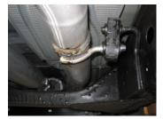
Next, install the headpipe #A. Insert welded hanger into rubber grommet. Use Factory clamp to secure together. DO NOT TIGHTEN.
