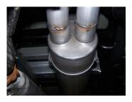
4. Install muffler #B onto headpipe #A 1.5-2" with the louvers facing towards the converter. Use a jack stand to support the muffler. Use clamp #I to secure the muffler to the headpipe. Do not tighten. Muffler inlet is looking into the louvers.
