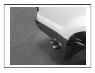
INSTALL YOUR STAINLESS TIPS. TIGHTEN ALL CLAMPS STARTING FROM THE FRONT, WORKING YOUR WAY TO THE BACK OF THE TRUCK. TO CLEAN TIPS USE A STAINLESS STEEL CLEANER & SCOTCH BTIE PAD.
