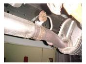
**1.** To remove the stock exhaust from the second clamp located in front of the stock muffler. Disengage the welded hangers using WD-40 from the OEM rubber grommets. Do not damage or remove the rubber grommets as you will re-use them to mount your new system. Now, cut off tailpipe and remove exhaust.
