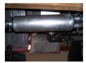
**3.** Install muffler #B onto head pipe #A  $1\frac{1}{2}$ "-2" with the louvers facing towards the converter. Use a jack stand to support the muffler. Use clamp #G to secure the muffler to the headpipe. Do not tighten. Muffler inlet is looking into the louvers.
