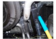
6. Install the passenger side overaxle tailpipe #F to the extension pipe. Use clamp #J to secure. Do not tighten. Insert welded hanger into rubber grommet.
