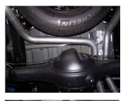
8. Install driver side overaxle tailpipe #G onto extension pipe, use clamp #J to secure pipe. Do not tighten. Insert welded hanger into rubber grommet.
