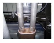
5. Install extension pipe #D into muffler. Use clamp #J to secure. Do not tighten. Next install driver side extension pipe #E into muffler using clamp #J to secure. Do not tighten. Insert welded hanger into rubber grommet.
