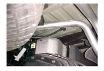
INSTALL DRIVERS SIDE TAILPIPE # D INTO MUFFLER  $1\frac{1}{2}$ " TO 2". INSERT WELDED HANGERS INTO RUBBER GROMMETS. USE CLAMP # H TO SECURE PIPE TO MUFFLER, DO NOT TIGHTEN.
