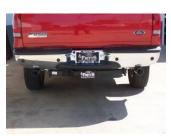
**8.** Install stainless steel tips. Clamp down. When you have everything in place, firmly tighten all bolts and clamps down securely. Use stainless steel cleaner and a Scotch Brite pad weekly to prevent tip from discoloration. Inspect all fasteners after 25-50 miles of operation and re-tighten as necessary
