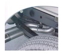
INSTALL DRIVERS SIDE TAILPIPE # D INTO MUFFLER 1 ½" TO 2". INSERT HANGER INTO RUBBER GROMMET, USE CLAMP # G TO SECURE PIPE TO MUFFLER. DO NOT TIGHTEN. THE TAB ON THIS PIPE SHOULD GO ON TOP OF PASSENGER SIDE PIPE USE BOLT KIT # J TO SECURE TOGETHER.
