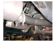
INSTALL FRONT MUFFLER HANGER # F ONTO MUFFLER INLLET, INSERT HANGER INTO RUBBER GROMMET, DO NOT TIGHTEN. USE BOLT KIT # I TO SECURE.
