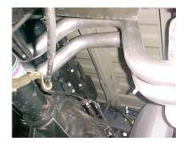
INSTALL PASS. SIDE TAILPIPE # C INTO MUFFLER 1  $\frac{1}{2}$ " TO 2". INSERT HANGER INTO RUBBER GROMMET, USE CLAMP # G TO SECURE PIPE TO MUFFLER. DO NOT TIGHTEN. YOU MAY NEED TO LOOSEN AND PUSH OVER TOWARDS THE DRIVERS SIDE AND RE-TIGHTEN.
