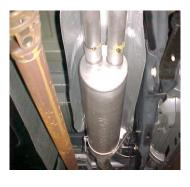
INSTALL MUFFLER # B ONTO HEADPIPE 1  $\frac{1}{2}$ " TO 2". USE CLAMP # F TO SECURE MUFFLER TO HEADPIPE. DO NOT TIGHTEN. USE A JACK STAND TO HOLD UP THE MUFFLER. OUTLETS SHOULD BE LEVEL.
