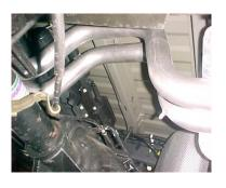
INSTALL PASS. SIDE TAILPIPE # C INTO MUFFLER 1 ½" TO 2". INSERT HANGER INTO RUBBER GROMMET, USE CLAMP # G TO SECURE PIPE TO MUFFLER. DO NOT TIGHTEN. YOU MAY NEED TO LOOSEN AND PUSH OVER TOWARDS THE DRIVERS SIDE AND RF-TIGHTEN.
