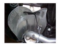
NEXT, REMOVE THE TWO BOLTS THAT HOLD THE HEAT SHIELD ON, THEN INSTALL THE REAR HANGER # E , RE-USING THE FACTORY BOLTS. ATTACH USING CLAMP # D.
