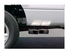
INSTALL STAINLESS TIPS, THEN TIGHTEN ALL NUTS, BOLTS, AND CLAMPS.
