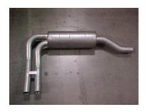
NEXT, INSTALL MUFFLER ASSEMBLY # A INTO STOCK HEADPIPE AND ATTACH WITH CLAMP # D.
