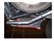
**8.** Next install the exit pipes #E. Use clamp #H to secure. DO NOT TIGHTEN.
