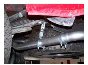
**6.** Install metal hanger #I into hole located approximately 19" from the rear of the frame in the second hole from top. Use bolt kit #J to secure. DO NOT TIGHTEN.
