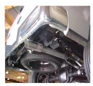
INSTALL EXIT PIPES # E ONTO TAILPIPES. ROTATE UNTIL LEVEL, USE CLAMP # H TO SECURE PIPES TOGETHER. DO NOT TIGHTEN.
