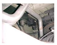
INSTALL DRIVERS SIDE TAILPIPE # D INTO MUFFLER 1 ½" TO 2". INSERT WELDED HANGERS INTO RUBBER GROMMETS. USE CLAMP # H TO SECURE PIPE TO MUFFLER, DO NOT TIGHTEN.
