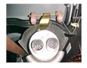
Install muffler #B onto head pipe 1  $\frac{1}{2}$ " to 2" with the louvers facing towards the converter. Use a jack stand to support the muffler. Use clamp #J to secure the muffler to the head pipe. Do not tighten. Outlets should be on the bottom.
