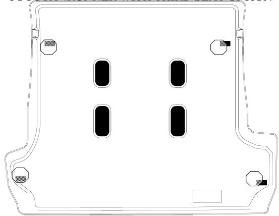
TO USE YOUR THIRD ROW FOLD DOWN SEATS WITH YOUR CARGO LINER IN PLACE, JUST TRIM AWAY THE MATERIAL FROM INSIDE OF THE FOUR (4) LARGE AREAS SHOWN ABOVE DARKENED. USE THE INSIDE EDGES OF THE PERIMETER RAISED BANDS AS A TRIMMING GUIDE. A PHOTO OF A TRIMMED PART IS SHOWN ON THE BACK OF THIS SHEET. <u>DO NOT USE THE THIRD SEATS WITHOUT FIRST TRIMMING YOUR CARGO LINER AS THE SEATS WILL NOT LOCK SECURELY INTO PLACE</u>.
