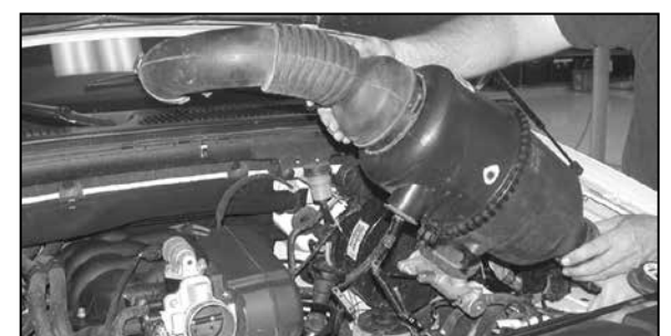
7. Remove the entire stock air intake assembly from the vehicle.
