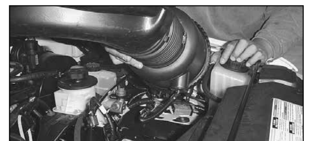
5. Detach the stock intake tube from the throttle body and lift up on the air cleaner assembly to release it from its retaining grommets.
