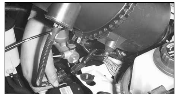
6. Disconnect the secondary mass air sensor electrical connection.
