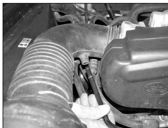
3. Disconnect the crank case vent from intake tube as shown.
