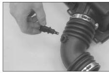
16. Carefully remove the air temperature sensor from the stock intake tube as shown.
