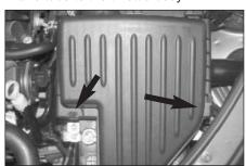
4. Unlatch the two air box lid retaining clips and remove the air box lid and intake tube from the vehicle.
