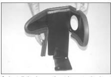
9. Install the long edge trim onto the heat shield as shown.
