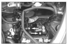
14. Install the heat shield onto the inserted nuts installed in step #13 and secure with the provided bolts and washers.
