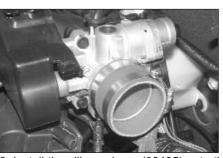
8. Install the silicone hose (08405) onto the throttle body and secure with the provided hose clamp as shown.
