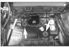
13. Install the two provided inserted nuts into the air box mounting plate as shown.
