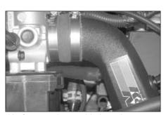
19. Connect the provided crank case vent hose onto the valve cover and then the K&N intake tube as shown.
