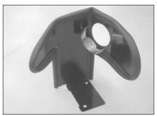
12. Install the saddle bracket assembly onto the heat shield as shown using the provided hardware.
