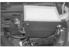
6. Pull up firmly on the air box base to dislodge it from the retaining grommets and then remove the air box from the vehicle.
