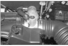
3. Loosen the hose clamp, which secures the intake tube to the throttle body.
