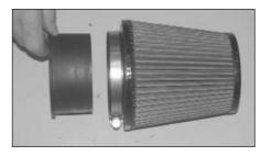
21. Install the provided filter adapter into the K&N filter as shown.
