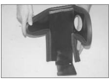
10. Install the short edge trim onto the heat shield as shown.
