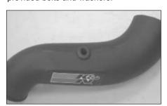
15. Install the provided grommet into the K&N intake tube as shown.
