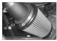
22. Install the K&N filter assembly onto the K&N intake tube, adjust the intake kit for the best fit and tighten all of the hose clamps.
