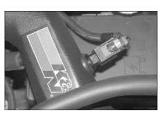
20. Reconnect the air temperature electrical connection.
