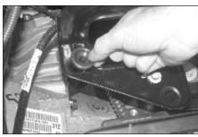
7. Remove the two air box retaining grommets from mounting tray as shown.
