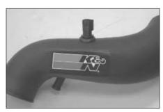
17. Install the air temperature sensor into the K&N intake tube as shown.
