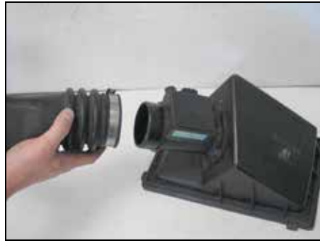
16. Loosen the hose clamp on the MAF sensor to disconnect the factory intake tube from the MAF sensor.
