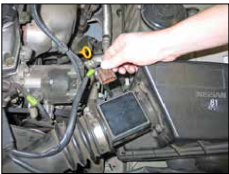
2. Disconnect the MAF sensor.
