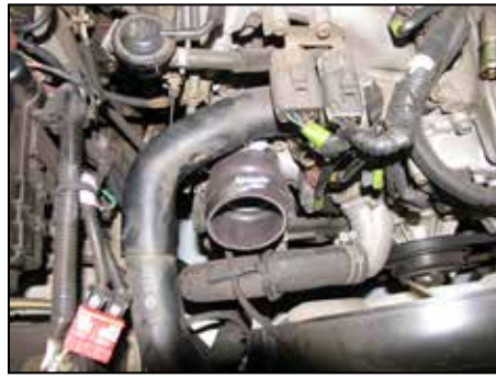
18. Attach the silicone hose with the provided hose clamps to the throttle body as shown.
