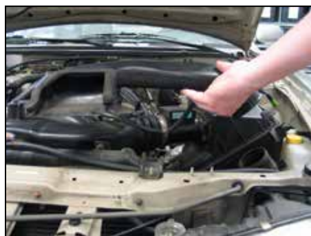
5. Firmly pull up to disconnect the fresh air inlet tube.
