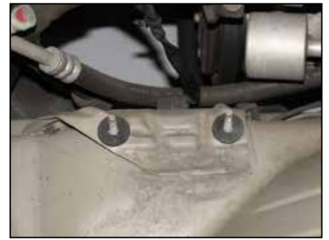
27. Install the provided rubber washers onto the lower air box mounting screws as shown.
