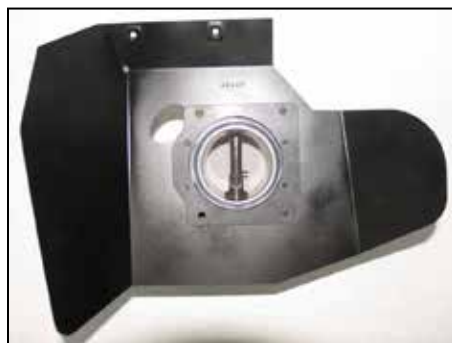
21. Place the 2nd provided gasket (10493) on the heat shield as shown.
