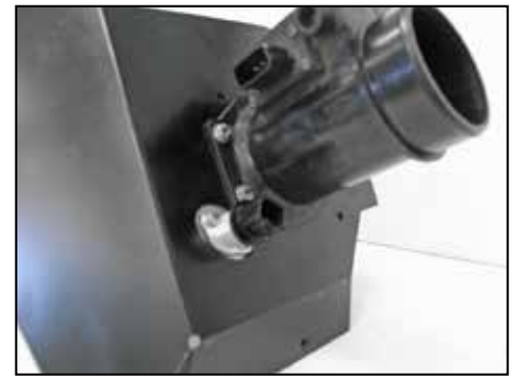
26. Attach the A/T sensor to the vent tube on the filter adapter.
