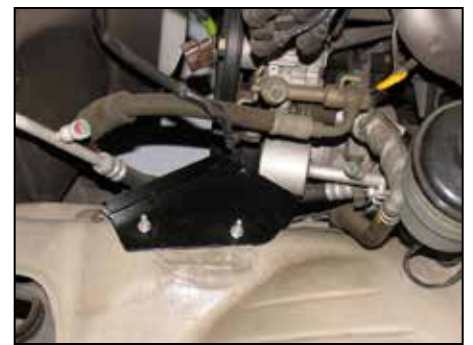
28. Install the bracket onto the mounting screws and then secure with the provided hardware.
