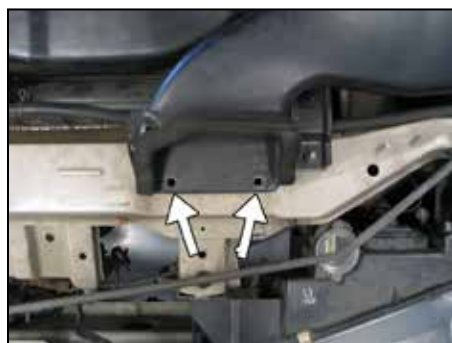
4. Remove the two clips that secure the fresh air inlet tube.
