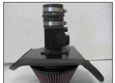
29. Attach the provided hose clamps and silicone hose to the air filter assembly as shown.
