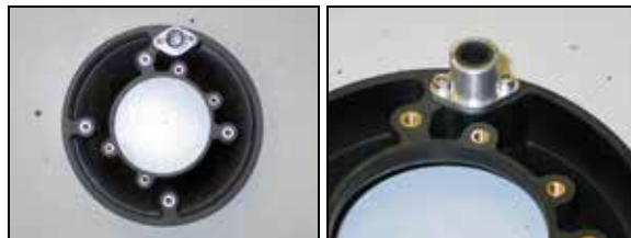
19. Place the provided gasket on the filter adapter, install the vent tube and secure with the hardware provided, and then install silicone hose onto vent tube.
