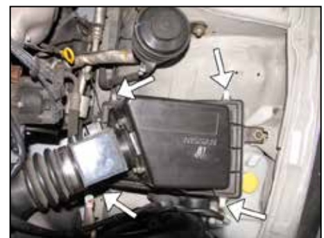
7. Unclip the four clips that secure the factory air box lid.
