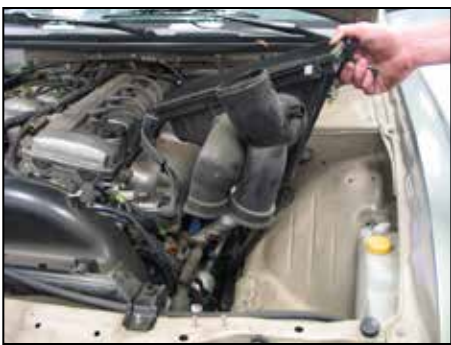
13. Pull up to remove the lower factory air box. NOTE: K&N Engineering, Inc., recommends that customers do not discard factory air intake.
