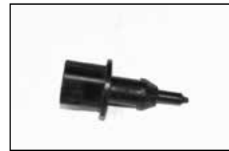
25. Remove the rubber grommet from the A/T sensor as shown.
