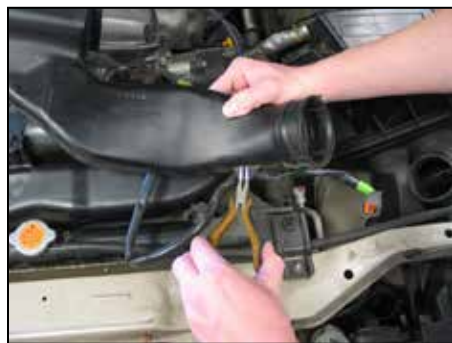
6. Turn the fresh air inlet tube upside down to unclip the A/T sensor wire harness.
