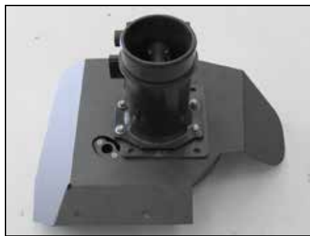
20. Place the heat shield on the MAF sensor as shown, with the gasket (10493) and 5mm hardware provided.
