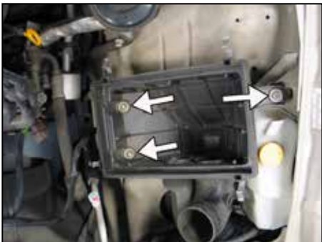
12. Remove the bolt and two nuts that secure the lower factory air box.
