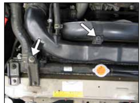
8. Loosen and remove the two bolts that secure the factory intake tube.
