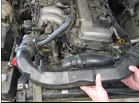
11. Remove the factory intake tube. NOTE: Unclip the vent hose from the intake kit.
