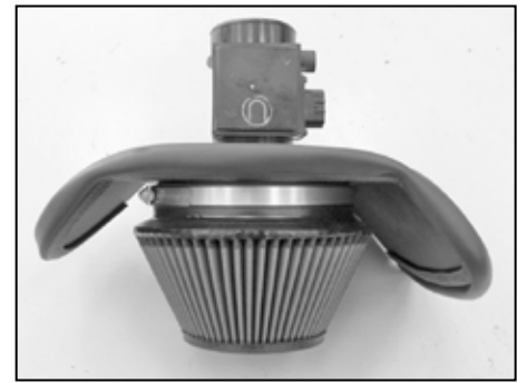
23. Attach the edge trim to the heat shield. It may be necessary to trim for proper fit.
