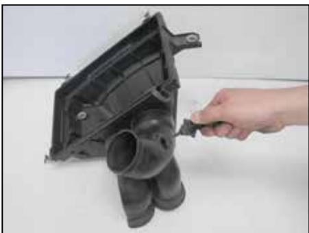
15. Remove the A/T sensor from the factory lower air box.
