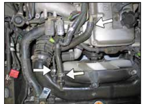
9. With pliers unclip the following hoses: the CCV hose, EGRC solenoid valve hose, and the vent hose.
