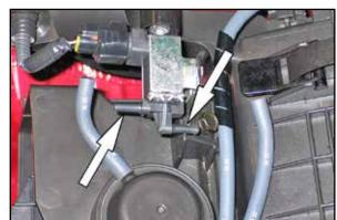
9. Disconnect the two vacuum lines from the secondary intake door vacuum switching valve.
