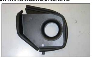
19. Install the filter adapter onto the heat shield and secure with the provided hardware.
