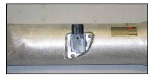
15. Install the mass air sensor into the K&N<sup>®</sup> intake tube and secure with the provided hardware.
