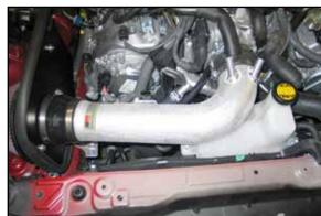
27. Install the K&N® intake tube into the silicone hose at the filter adapter, then into the silicone hose at the throttle body. Secure with the provided hose clamps.
