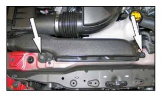
4. Pop up the center of the fresh air intake scoop retainer and remove the retainer. Remove the fresh air intake scoop retaining bolt and remove the fresh air scoop from the vehicle.
