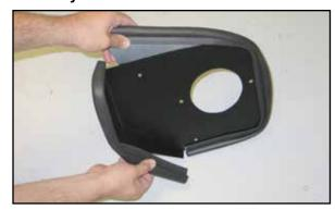
17. Install the short edge trim onto the heat shield as shown.
