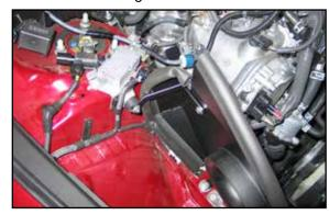
23. Install the heat shield mounting bracket (070112) onto the rubber mounting stud and then secure it to the heat shield with the provided hardware.
