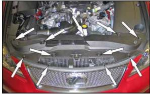
3. Pop up the centers of the nine front cover fasteners and remove the fasteners. Remove the front cover from the vehicle.
