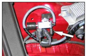
32. Install the vacuum plug onto the open port of the secondary intake door vacuum switch as shown.
