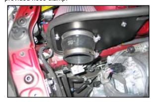
25. Install the silicone hose (08050) onto the filter adapter as shown and secure with the provided hose clamp.
