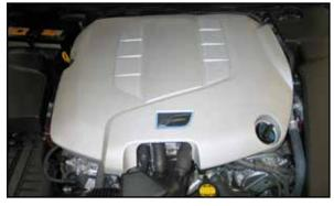
2. Lift up the engine cover to dislodge it from the mounting grommets and remove it from the engine.
