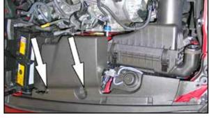
5. Pop up the centers of the strut tower cover retainer clips and remove the retainer clips. Loosen the strut tower cover retaining nut and then remove the strut tower cover.
