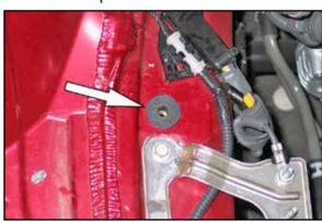
20. Install the inserted nut into the air box mounting grommet hole in the inner fender as shown.
