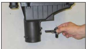
14. Remove the mass air sensor from the factory air box as shown.
