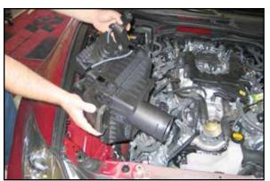
12. Lift up the air box to gain access to the remaining vacuum line connection and wiring harness clip. Disconnect the vacuum line and unhook the wiring harness from the air box. Remove the air box from from the vehicle.
