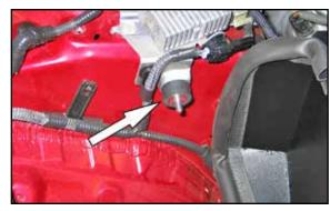
22. Install the provided rubber mounted stud into the module mounting bracket as shown.
