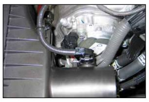
8. Disconnect the mass air sensor electrical connection and unhook the wiring harness from the air box.
