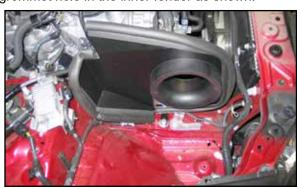
21. Install the heat shield assembly and secure the mounting bracket to the inserted nut installed in the previous step.
