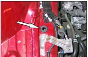
13. Remove the air box mounting grommet shown from the inner fender.
