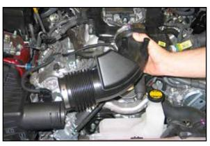
7. Loosen the two hose clamps, which secure the intake tube to the throttle body and air box. Then remove the intake tube from the vehicle.
