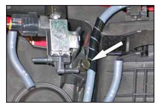
10. Remove the bolt which secures the secondary intake door vacuum switching valve to the air box. **NOTE: This bolt will be reused in a later step.**
