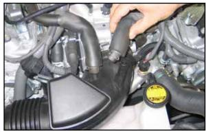
6. Loosen the two spring clamps that secure the crank case vent hoses to the intake tube. Then disconnect the crank case vent tubes from the intake tube.
