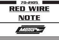
The 70-2105 comes with both a red wire in the harness and also a loose red wire. **The red wire in the harness will only be used in the 2007 CHEVROLET AVEO.** All other applications will tape off the red wire in the harness and use the loose red wire supplied. You must run one end of the loose red wire to a 12 volt accessory wire or fuse either under the steering column or fuse box, and the other end to the aftermarket radios 12 volt accessory lead.
