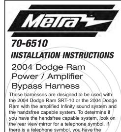
the rear view mirror for a telephone symbol. If there is a telephone symbol, you have the handsfree system, if not please refer to the 70-6512, 2002-04 Dodge Ram power/amp bypass harnesses. A power harness is supplied to allow the user to wire up the aftermarket radio without the need to purchase any other harnesses.
