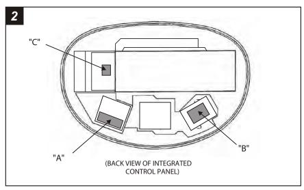
Turn the integrated control panel over and disconnect the vent control harness ("A"), fan speed control harness ("B"), and defroster harness ("C"). Unclip the main switch harness from the side of the factory unit. (This harness connects the fan speed control harness, vent control harness and defroster harness).
