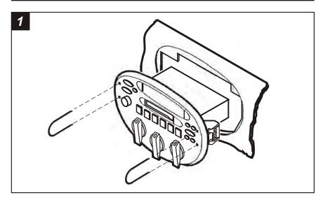
Disconnect the negative battery terminal to prevent an accidental short circuit. Reach under the driver's side dash and unclip the temperature control cable. Using Metra's 86-5618, pull the factory radio/climate control panel from the dash. Disconnect the switch power harness, antenna plug, radio/speaker power harnesses and vacuum hose harness.
