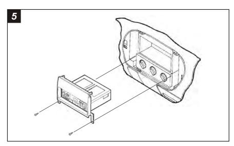
Re-connect the battery terminal and test the unit for proper operation. Remove the top (2) Phillips screws securing the climate control cluster to the sub-dash. Slide the head unit/kit assembly into the dash cavity (be sure the *Rear Support Bracket* engages the support shelf in the dash). Mount the bottom legs of the kit to the same holes in the climate control cluster with the (2) Phillips screws previously removed.
