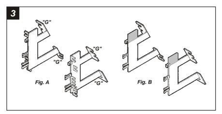
Cut and remove all mounting tabs on **Bracket Set #2** EXCEPT tabs **"G"**. The mounting tabs can be identified by the stamped letter on the back of each tab. (see Fig. A). Once the mounting tabs are removed, cut and remove the SHADED portions of the Brackets. (see Fig. B). Skip to the Installation Instructions for ALL VEHICLES on Page #12.
