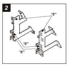
Cut and remove mounting tabs "A" and "B" on the **Radio Housing.** Cut and remove all mounting tabs on **Bracket Set #2** EXCEPT tabs "E". The mounting tabs can be identified by the stamped letter on the back of each tab.
