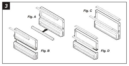
**DASH TRIM BEZELS WITH A DIVIDED RADIO OPENING:** If keeping the factory pocket is NOT desired, cut and remove the upper rib from the radio openingand snap the **Filler Bar** onto the bottom of the **Radio Housing.** (see Fig. A). If keeping the factory pocket is desired, cut and remove the upper rib from the radio opening and the bottom portion of the **Radio Housing.** (see Fig. B). Skip to the Installation Instructions for ALL VEHICLES on Page #12.
