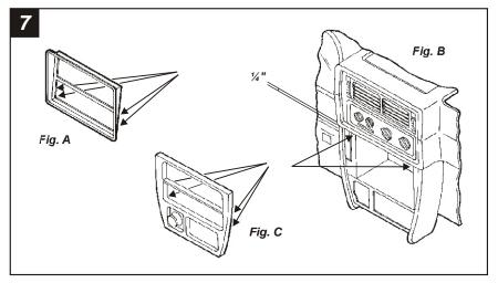
TALON 1995-98, ECLIPSE 1995-98, COLT, SUMMIT, MIRAGE, STEALTH, 3000GT, DIAMANTE, GALANT, MONTERO: No cutting of the dash or dash trim bezel is required. Skip to the Wiring Preparation in step #8.
