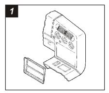
Disconnect the negative battery terminal to prevent an accidental short circuit. Unclip the radio trim bezel (the factory pocket will be attached). Remove (4) screws securing the factory head unit and disconnect the wiring.
