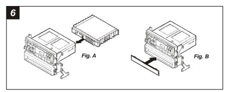
**IF AN EQUALIZER WILL BE INCLUDED:** Slide the aftermarket equalizer into the back of the **Radio Housing.** Using the hardware included with the equalizer, mount the unit to the kit. (see Fig. A)
