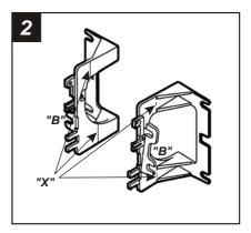
Cut and remove mounting tabs "A" and "B" on the **Radio Housing**. Locate mounting tabs "B" on **Bracket Set #3** and cut and remove the mounting legs containing tabs "A" by cutting along scored lines "X". The mounting tabs can be identified by the stamped letter on the back of each tab.
