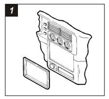
Disconnect the negative battery terminal to prevent an accidental short circuit. Unclip the radio/climate control trim bezel and remove the bezel. Remove (4) Phillips securing the factory head unit and disconnect the wiring.
