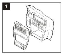
Disconnect the negative battery terminal to prevent an accidental short circuit. Pry out on the top of the dash trim bezel and remove the bezel. Remove (4) screws securing the factory head unit and disconnect the wiring.
