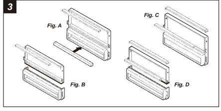
**DASH TRIM BEZELS WITH A DIVIDED RADIO OPENING:** If keeping the factory pocket is NOT desired, cut and remove the upper rib from the radio openingand snap the **Filler Bar** onto the bottom of the **Radio Housing.** (see Fig. A). If keeping the factory pocket is desired, cut and remove the upper rib from the radio opening and the bottom portion of the **Radio Housing.** (see Fig. B). Skip to the Installation Instructions for ALL VEHICLES on Page #12.
