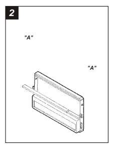
Cut and remove all mounting tabs on the *Radio Housing* EXCEPT tabs "*A*". The mounting tabs can be identified by the stamped letter on the back of each tab. (*Fig. A*). Cut and remove the *lower* rib from the radio opening. (*Fig. B*)
