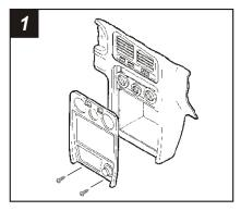
Disconnect the negative battery terminal to prevent an accidental short circuit. Unclip the gear shifter trim panel and remove. Remove (2) Phillips screws exposed at the base of the dash trim bezel. Unclip the dash trim bezel. Remove (4) Phillips screws securing the factory head unit and disconnect the wiring.
