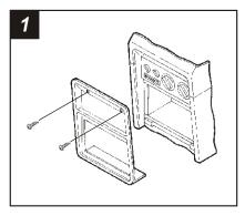
Disconnect the negative battery terminal to prevent an accidental short circuit. Remove (2) screws above the climate controls. Unclip the bottom of the dash trim bezel and remove the bezel. Remove (4) screws securing the factory head unit and disconnect the wiring.
