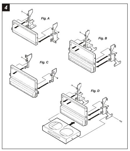
IF THE LOWER PORTION OF THE RADIO HOUSING HAS BEEN REMOVED FOR POCKET RETENTION: Mount the Brackets to the Radio Housing with (2) clips and (2) #6 x %"Phillips Flat-head Screws supplied. (see Fig. A)
