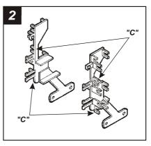
Cut and remove mounting tabs "A" and "B" on the **Radio Housing.** Locate mounting tabs "C" on **Bracket Set #1.** The mounting tabs can be identified by the stamped letter on the back of each tab.
