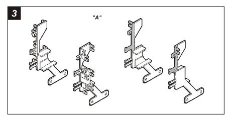
Cut and remove all mounting tabs on **Bracket Set #1** EXCEPT tabs "**A**". The mounting tabs can be identified by the stamped letter on the back of each tab. (see Fig. A). Once the mounting tabs are removed, cut the SHADED portions from the Brackets. (see Fig. B). (The SHADED portions of the Brackets will be mounted to the **Radio Housing** in step #4). Skip to the Installation Instructions for ALL VEHICLES on Page #12.
