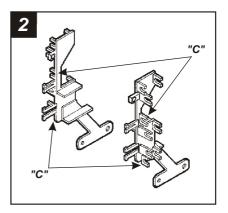
Cut and remove mounting tabs "A" and "B" on the **Radio Housing**. Cut and remove all mounting tabs on **Bracket Set #1** EXCEPT tabs "C". The mounting tabs can be identified by the stamped letter on the back of each tab.
