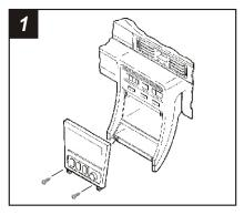
Disconnect the negative battery terminal to prevent an accidental short circuit. Remove (2) Phillips screws from each side of the gear shifter console. Remove (2) Phillips screws from the top of the console (under the ashtray). Lift the console out and remove (2) Phillips screws exposed at the base of the dash trim bezel. Pull out on the bottom of the dash trim bezel, disconnect the wiring and remove the bezel. Remove (4) screws securing the factory head unit and disconnect the wiring.
