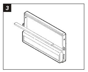
Cut and remove the *lower* rib from the radio opening. *Skip to the Installation Instructions for ALL VEHICLES on Page #12.*
