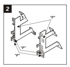
Cut and remove mounting tabs "A" and "B" on the **Radio Housing**. Cut and remove all mounting tabs on **Bracket Set #2** EXCEPT tabs "F". The mounting tabs can be identified by the stamped letter on the back of each tab.
