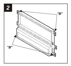
Cut and remove all mounting tabs on the **Radio Housing** EXCEPT tabs **"B".** The mounting tabs can be identified by the stamped letter on the back of each tab.
