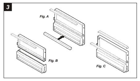
**DASH TRIM BEZELS WITH A DIVIDED RADIO OPENING:** If keeping the factory pocket is NOT desired, cut and remove the upper rib from the radio openingand snap the **Filler Bar** onto the bottom of the **Radio Housing.** (see Fig. A). If keeping the factory pocket is desired, cut and remove the upper rib from the radio opening and the bottom portion of the **Radio Housing.** (see Fig. B). Skip to the Installation Instructions for ALL VEHICLES on Page #12.
