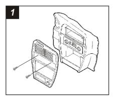
Disconnect the negative battery terminal to prevent an accidental short circuit. Remove (2) Phillips screws below the a/c vents. Pry out on the top of the dash trim bezel and remove the bezel. Remove (4) screws securing the factory head unit and disconnect the wiring.
