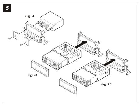
**2-SHAFT HEAD UNITS:** Snap the **Shaft Supports** into the **Radio Housing.** Slide the aftermarket head unit into the kit and secure with shaft nuts. (see Fig. A).
