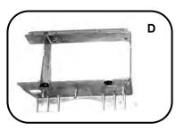
4 Slide radio bracket off of radio.
