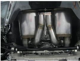
**Step 4.** Now you can re-attatch the rear valance to the vehicle using the OEM fasteners. Once the rear valance is back in place loosely attach the Tip assembly to the Muffler assemblies using the provided 2.50" clamps.
