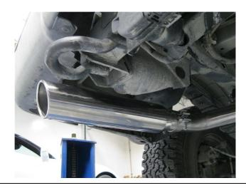
MAGNAFLOW: 22961 Arroyo Vista - Rancho Santa Margarita, CA 92688 | 1(800) 990-0905 Technical Support: 1(800) 959-9226 | Email: moreinfo@magnaflow.com **Step 4.** Lastly, install the tips to the Tail pipe Assemblies using the supplied 2.50" clamps. The supplied adjustable tips are design to fit a variety of aftermarket bumpers and rollpans, once a position is decided for the tips it is recommended to have them welded into place.
