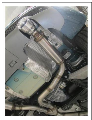
**Step 4.** Next install the P/S Muffler Assembly in similar fashion as the D/S using the supplied 2.50" clamp and inserting the hanger in to the rubber insulator.
