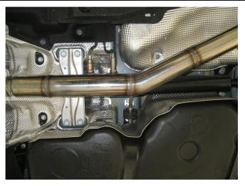
**Step 2.** Begin installation of your new MAGNAFLOW exhaust system by attaching the Y-Pipe Assembly to the resonator outlet using the OEM clamp. Insert the hanger into OEM rubber insulators and re-install the O2 sensors.
