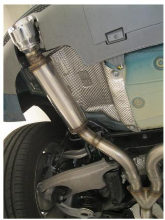
**Step 3.** Then install D/S Muffler Assembly in a similar fashion as the Y-Pipe assembly using the supplied 2.50" clamp and inserting the hanger into the OEM rubber insulaters.
