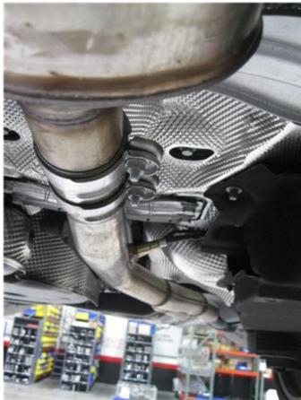
**Step 1.** Start by removing the O2 sensors from the pipe behind the resonator. Loosen the OEM clamp behind the resonator. Disengage the exhaust hangers from the rubber insulators (Save the insulators and clamp as they will be re-used on the new system), and remove the exhaust system.
