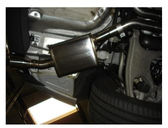
**Step 3.** Next Install the Muffler Assemblies to the outlets of the Resonator Assembly using the supplied 2.50" clamps. Insert hangers into rubber insulators.
