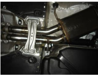
**Step 2.** Begin installation of the new system by fastening the Resonator Assembly inlet to the catalytic converter using the OEM clamps and fitting the hangers into the rubber insulators (Leave all clamps and fasteners loose for final adjustment of the complete system.)
