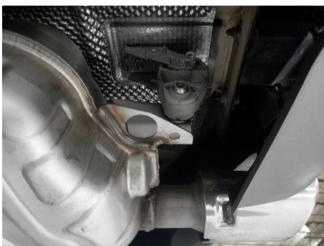
**Step 1.** To extract the OEM exhaust system it is necessary to remove the underbody braces on the rear of the vehicle. Begin removing the exhaust by un-fastening the front clamps located behind the catalytic converters. Next, with the exhaust supported, work rearward and disengage all welded hangers from the rubber insulators. Do not damage or discard the rubber insulators or clamps as they will be re-used to mount the new system. You can now remove the exhaust from the vehicle.
