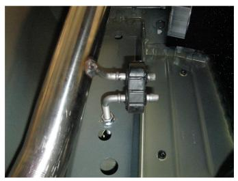
**Step 5.** For the passengers side Tail Pipe Assembly there is an existing hole in the vehicles sub frame. The hole location will be apparent once the Tail Pipe Assembly is in position. Locate the supplied threaded hanger and hardware. Use the suppled rubber insulator to attach the welded hanger on the pipe as shown.
