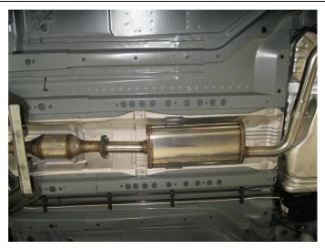
**Step 3.** Install the new system by attaching the Muffler Assembly to the OEM catalytic converter outlet pipe using the OEM bolts and supplied hardware. Leave all clamps and fasteners loose for final adjustment of the complete system once installed.
