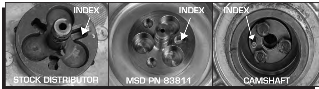
Figure 1 The Drive Mechanism of the PN 83811 Distributor.
