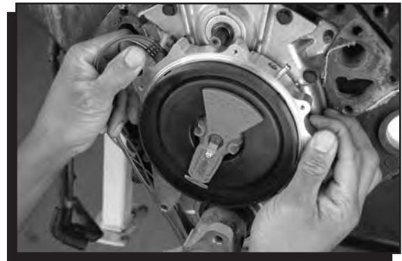
Figure 11 Installing the New Distributor.
