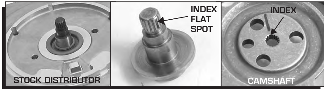
Figure 1 The Drive Mechanism of the PN 8381 Distributor.
