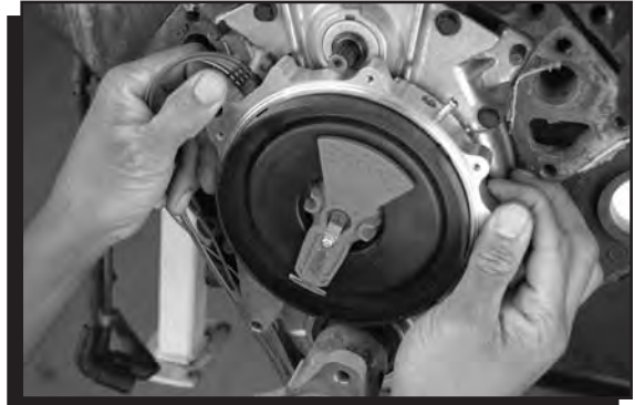
Figure 9 Installing the New Distributor.
