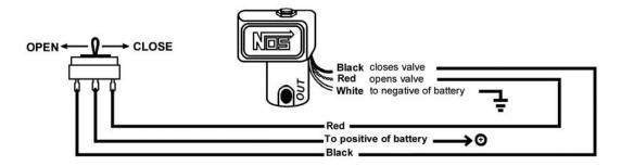
NOTE: Install the Remote Electronic Control Bottle Valve onto the bottle valve tightly and wire the switch as shown above.
