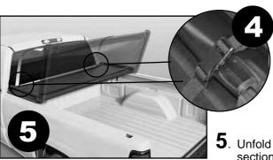
4. Undo both clips so cover can be unfolded.
