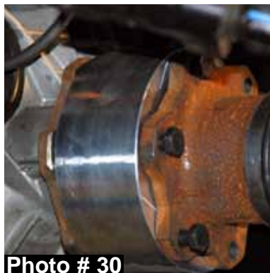
Driver side shown with 3.35" cv-shaft spacer.
