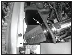
Step 19 Install the filter and fully tighten the clamp.
