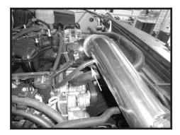
Step 18 Install the new hose onto the vacuum fitting on the intake tube.
