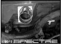
Step 12 Install the supplied firewall mount and secure with the three supplied self tapping screws.
