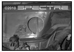
Step 11 Drill three 1/8" holes at each of these locations that you traced.
