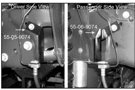
secure the brake hoses to the frame; these brackets were unbolted from the frame during disassembly. Completely remove the frame-mounting bracket from the brake hose by removing the horseshoe clip. Gently loosen the fitting between the hard line and the rubber hose just enough to rotate the hose so that it is pointing downward.
