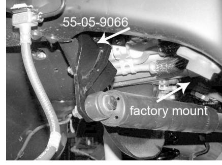
The rubber brake hose's lower end, and the 4WD activation vacuum line, are attached to the front axle via a bracket located in front of the coil spring's lower seat. Unplug the vacuum line where it passes through this bracket then unbolt the bracket from the axle.
