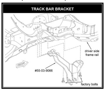
□ [SEE DIAGRAM] Position the Superlift® track bar spacer (#55-01-9074) between the track bar bracket (#55-03-9066) on the frame on the rear hole in the factory location, and secure using the five factory bolts (136).
