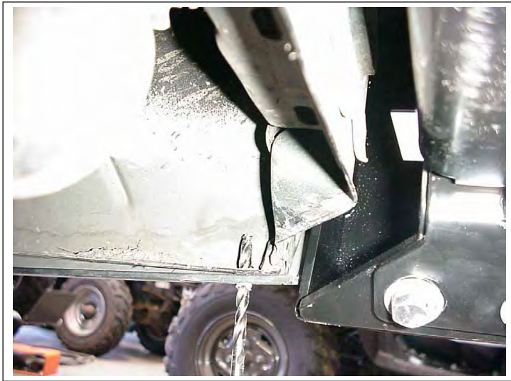
Figure 8A, Drill Hole in Plastic Side Fender Skirting
