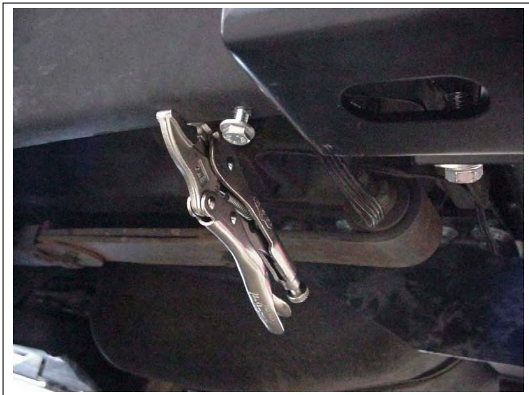
Figure 8B, Bolt Bottom Rear of Plastic Side Fender Skirting
