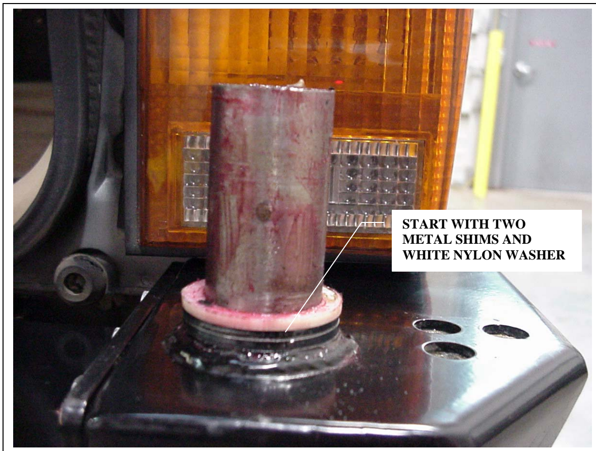
Figure 10A, Shims on post
