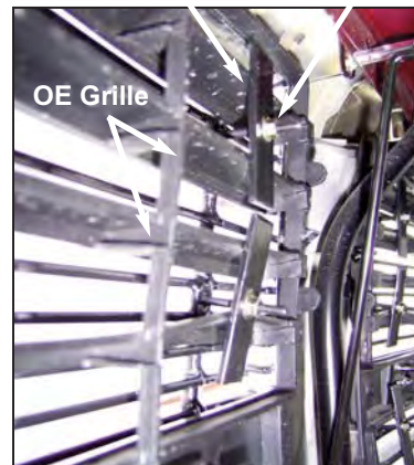
FIGURE 2 - BRACKETS/M4 FLANGE NUTS
