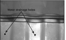
Water drainage holes on floor behind cab. Seal with silicon if desired.
