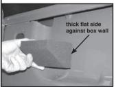
use 1 small foam wedge positioned as shown. Thick side against box wall.
