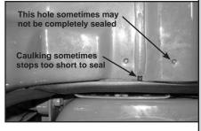
Sometimes hole is not sealed on floor and OEM caulking sometimes stops short at end of box. Seal with silicon if desired.
