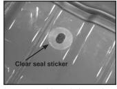
a) At tailgate end locate round b) Locate oblong hole on box floor behind cab. Wipe with alcohol. Apply clear seal sticker over hole.
