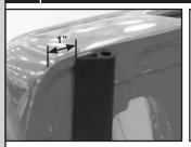
At top of box, by tailgate (makes sure area is still clean) start applying TrailSeal 1" back as shown above.
