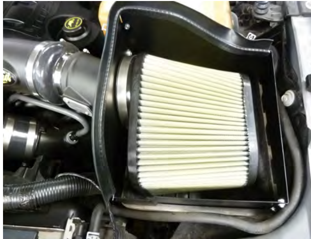
14. Install the Airaid Premium Filter onto the Sensor Tube and tighten the clamp.
