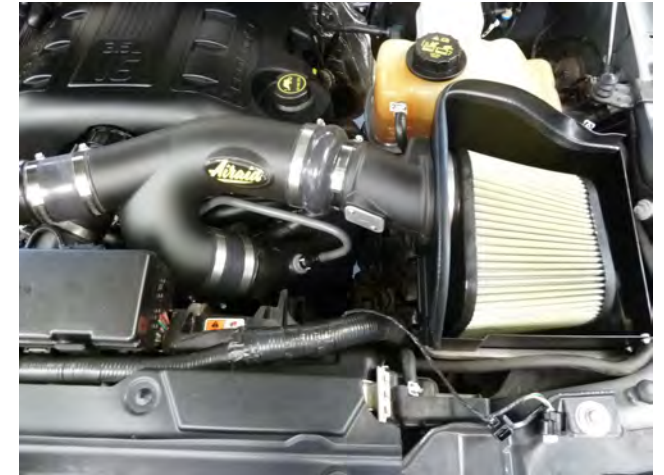
15. Double check your work. Make sure there is no foreign material in the intake path. Make sure all clamps, hoses, bolts, and screws are tight. Double check the hood clearance. Reconnect the negative battery cable.
