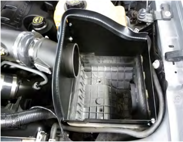
13. Tighten the Clamps on the Hump Hose, reconnect the MAF or MAP sensor and install the Weather Strip as shown, with the contour rolling away from the Filter area.
