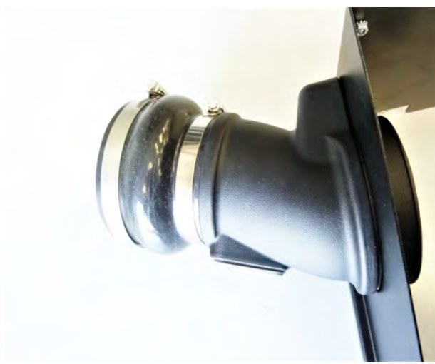
11. Slide the Hump Hose and Clamps onto the Sensor Tube as shown.
