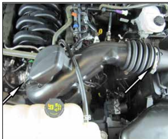
2. Loosen the intake clamps on the throttle body and the air box outlet.
