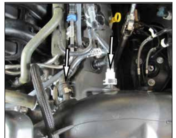
3. Disconnect the two breather lines and remove the intake tube from the vehicle.
