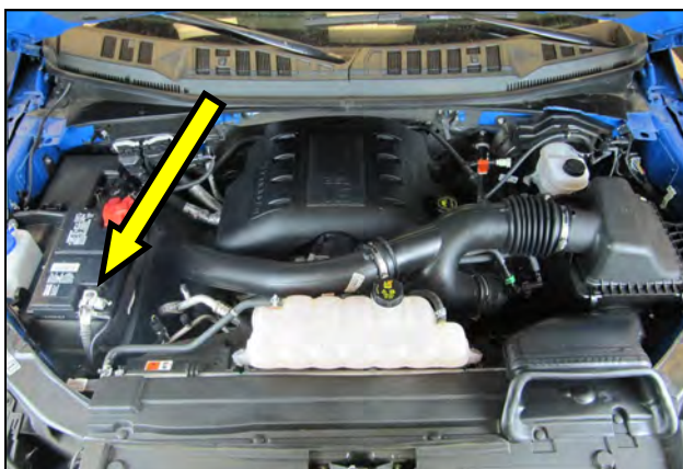
1. Disconnect the negative battery terminal.
