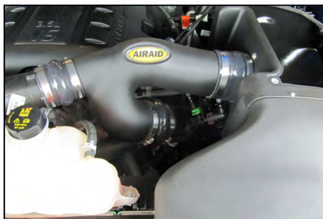
17. Connect the Airaid Intake Tube onto the factory turbo plumbing, then into the Air box Coupler. Rotate the Tube forwards and backwards until proper alignment is achieved and tighten all six Clamps.
