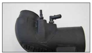
15. Install the provided vent fittings into the AIRAID® intake tube as shown.
