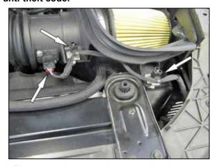
2. Disconnect the mass air sensor electrical connection and then unhook the harness retaining clips.
