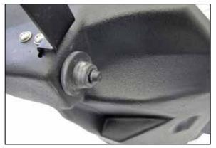
8. Install the factory air box mounting bracket onto the mounting stud installed onto the AIRAID® air filter housing in the previous step.
