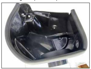
9. Install the provided edge trim onto the AIRAID® filter housing as shown.
