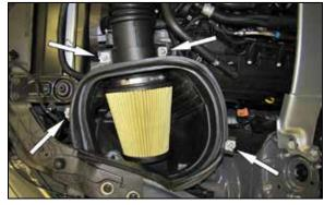
3. Remove the four nuts that secure the upper half of the factory heat shield and lip seal.
