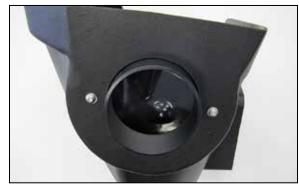
6. Install the provided filter adapter into the AIRAID® filter housing and secure with the provided hardware.
