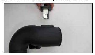
14. Install the mass air sensor assembly into the AIRAID® intake and secure with the provided hardware.
