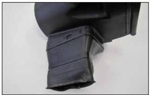
10. Remove the fresh air intake duct from the factory air filter housing and install it onto the AIRAID® air filter housing.
