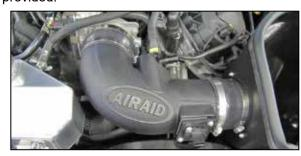
17. Install the AIRAID® intake tube into the coupler at the heat shield and then the throttle body, adjust the tube for best fit and then secure with the provided hose clamps.
