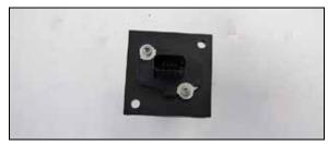
13. Install the provided gasket onto the mass air sensor adapter. Remove the mass air sensor from the factory hosing and install it into the AIRAID® adapter and secure with the provided hardware.
