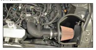
19. Connect the factory vent lines to the fittings installed into the AIRAID® intake tube.
