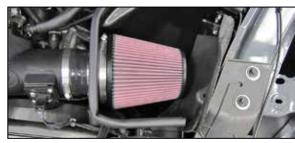
18. Install the AIRAID® air filter onto the filter adapter and secure with the provided hose clamp. Reconnect the mass air sensor electrical connection.
