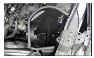
11. Install the AIRAID® filter housing assembly into the vehicle and secure with the factory bolt used to secure the factory housing.
