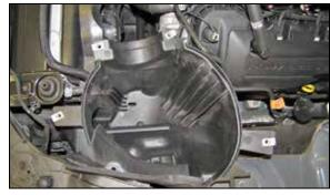
5. Remove the foam air dam, then remove the bolt that secures the factory lower air filter housing and then remove the housing from the vehicle.
